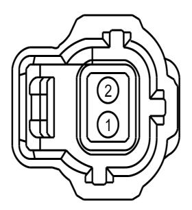
PinCircuitGaugeCircuit FunctionQualifier1134 (GY-OG)20Intermediate Shaft Speed (ISS) sensor, signal
